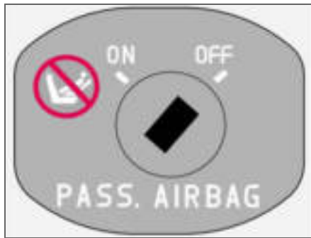
Switch for SRS in OFF position.
